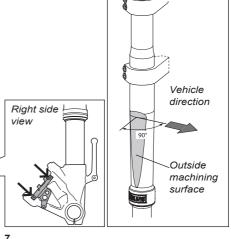
Tighten the triple clamp screws, refer to the vehicle service manual
