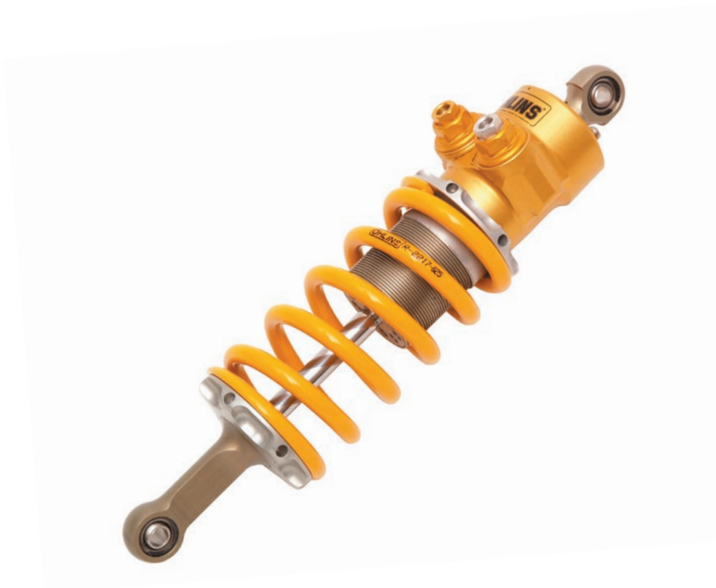
Figure 1.1 A complete TTX damper with spring
